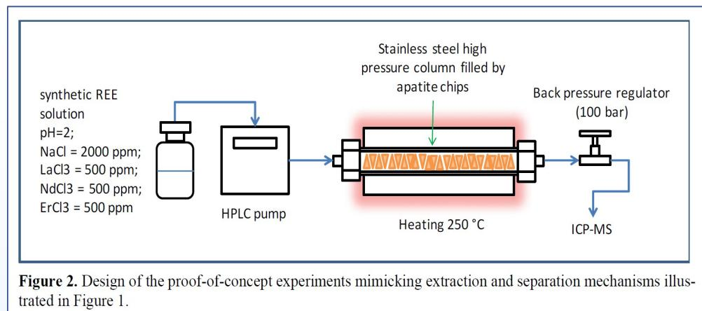
**Figure 2.** Design of the proof-of-concept experiments mimicking extraction and separation mechanisms illustrated in Figure 1.
