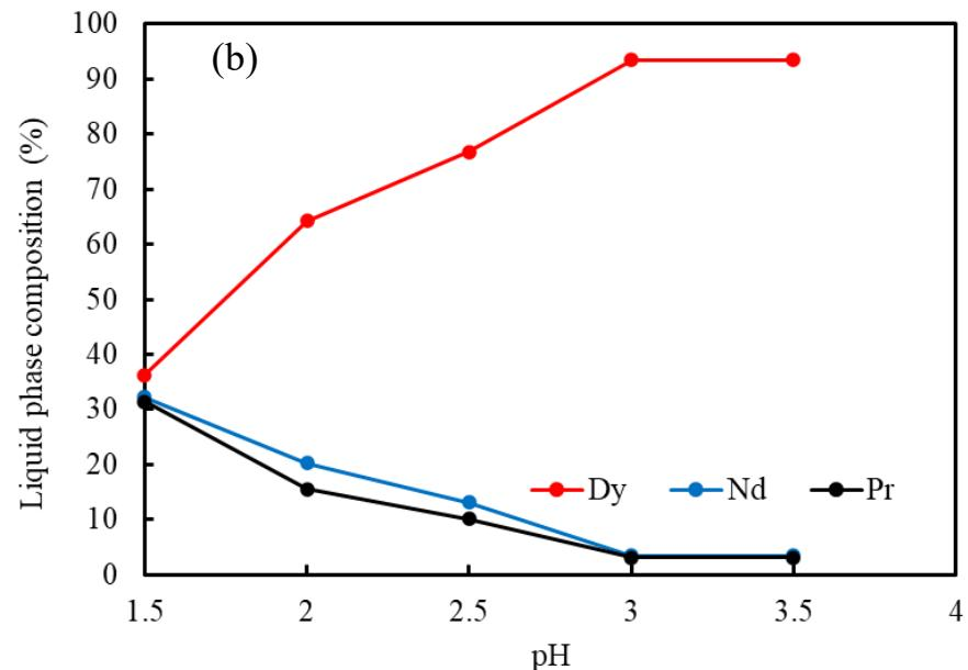
Effect of pH on (a) adsorption (%), (b) composition in the liquid phase (%).
