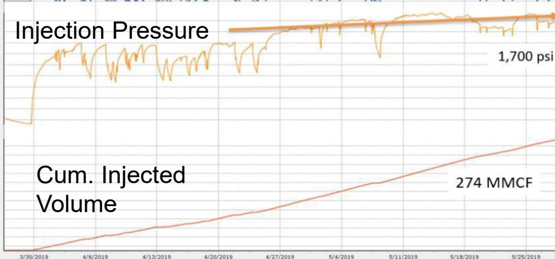
Injected gas quickly spread through field, evidenced by elevated gas production in offset wells, 7 hz wells shut in due to gas breakthrough, increased gas production noted more than mile away from injector
