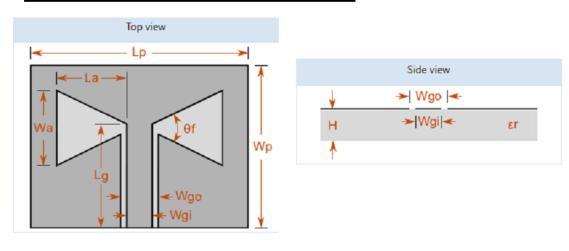
Antenna design parameters using Antenna Magus and CST Microwave Studio®.
