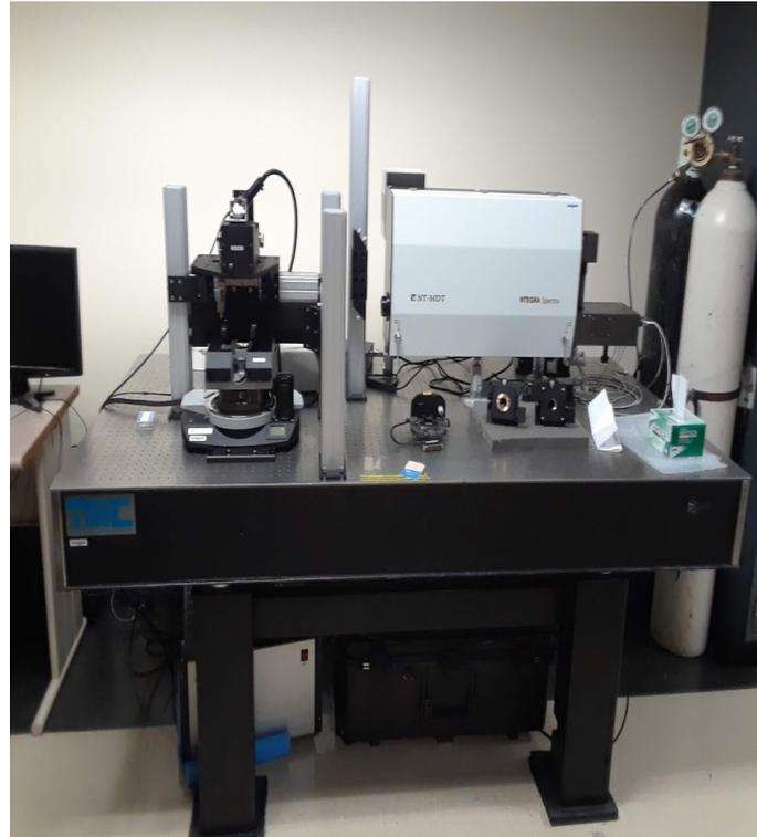
Integrated setup for SPM and Raman characterization
