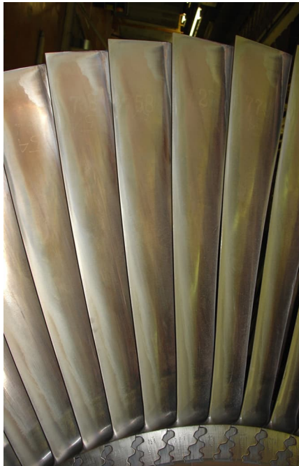
Water droplet induced blade root cracking for L0 blades in steam turbine
