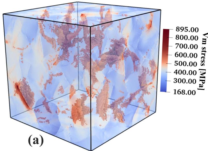
Hotspots in Ni microstructure after uniaxial deformation to 2.5% strain
