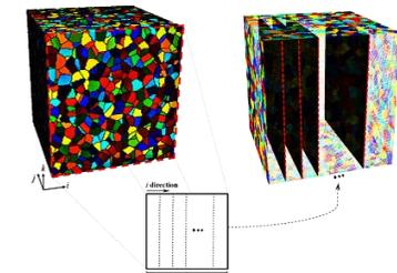
Domain decomposition of material microstructure for hybrid Multi-CPU/GPU accelerated simulation
