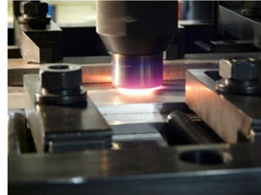
FSW of High Melting Point Material at PNNL
