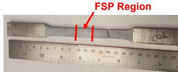
Room Temperature Tensile Test Coupon
