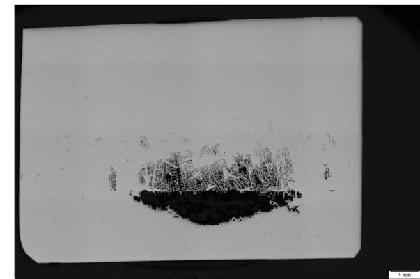
**Cast Plate Microstructure in Area of Porosity**
