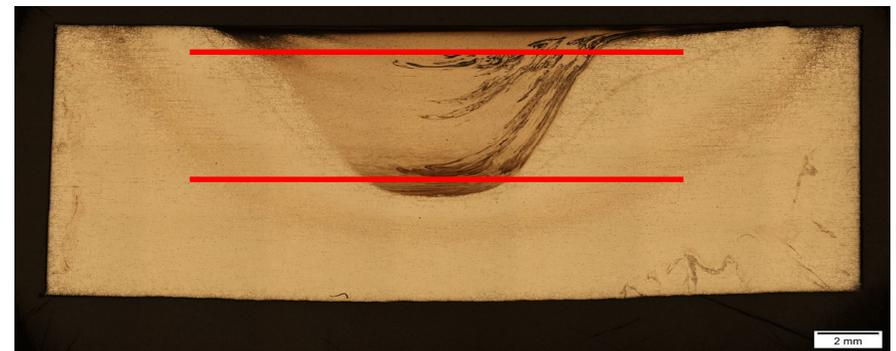
Creep Testing Coupon Material Area
