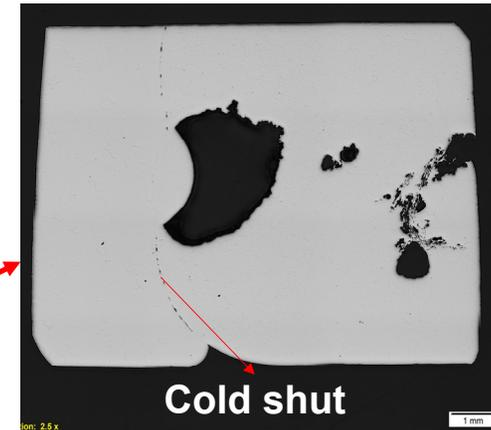
**Cast Plate Microstructure in Area of Cold Shut**
