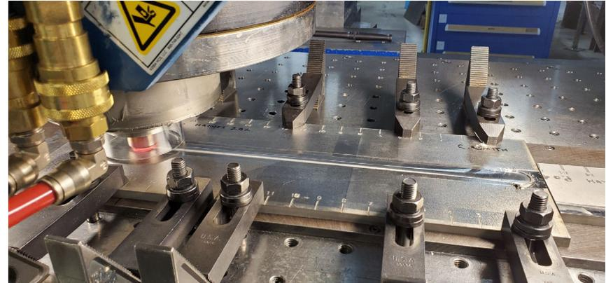
**FSP of Laser Ablated Material in Process**
