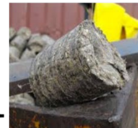
Densified biomass with less water uptake
