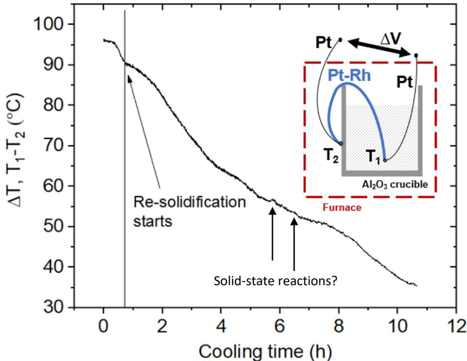
+ 2.4 °C/min cooling from 1600 °C (furnace T).
