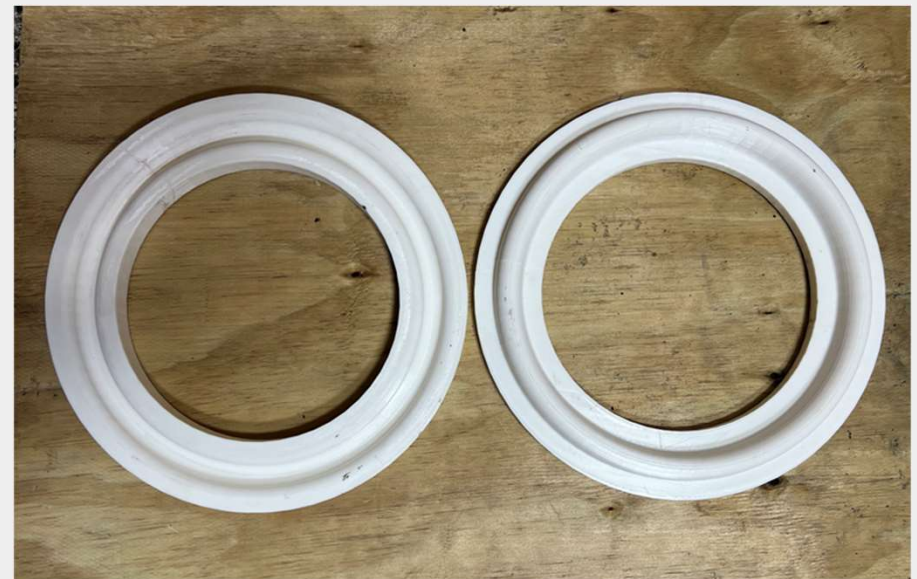
3D-Printed Prototype of mold inserts for Interlocking Mechanism
