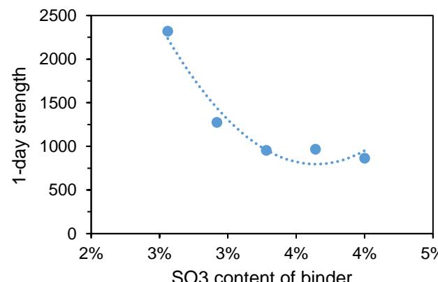
**ASTM - C563:** Standard Guide For Approximation of Optimum  $\text{SO}_3$  in Hydraulic Cement.
