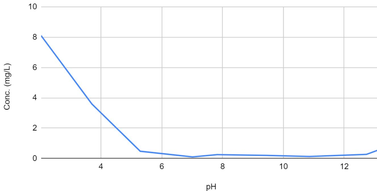
Chromium concentration from EPA Method 1313 for **fresh Class F Fly Ash sample.**
