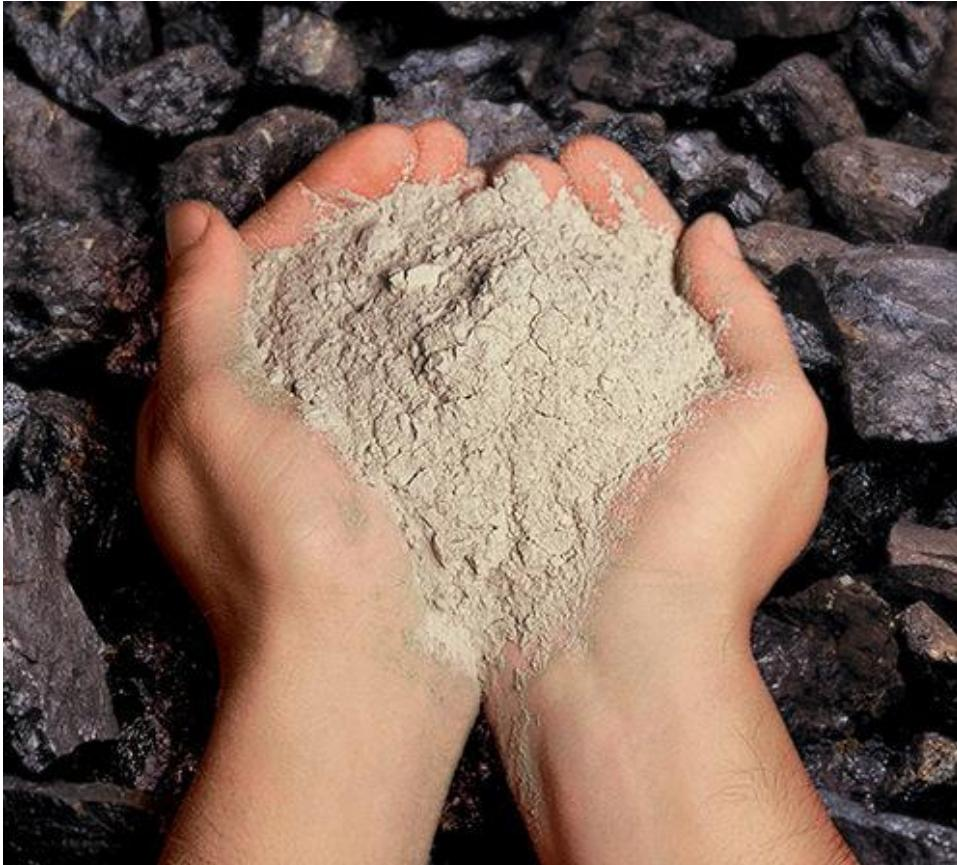
FA particles carried out of coal combustion chamber by exhaust gases and subsequently filtered out
