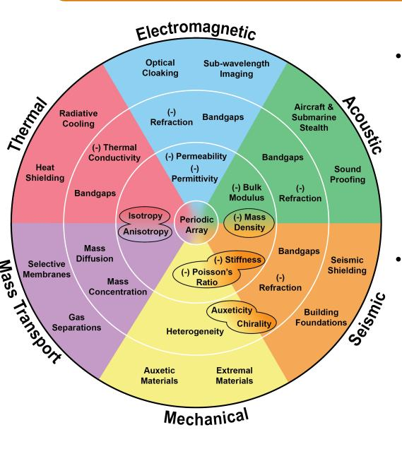
Metamaterials are artificial materials composed of unit cells that work collectively to produce unusual, unique physical properties not found in natural materials or traditional composite materials
