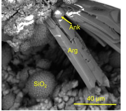
Amorphous silica is also proximal to the carbonate nodule (Ank) and aragonite (Arg) intergrowths. PNNL forced oscillation testing of injectable contrast agent nanofluids used to parameterize forward seismic modeling
