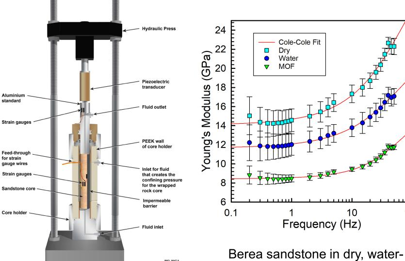
Forced oscillation apparatus for measuring the elastic properties (Young's modulus, E) and extensional attenuation (Q<sup>-1</sup><sub>F</sub>) in Berea sandstone
