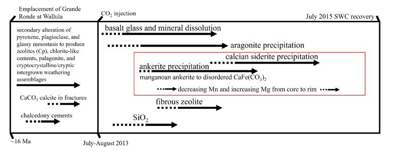
Overall mineralization paragenesis for the Grande Ronde basalt at the Wallula Basalt Carbon Storage Pilot Project. Dashed arrows denote uncertain initiation and duration. The red-framed box specifies that the compositions of the carbonate precipitates are consistent with ankerite and siderite.
