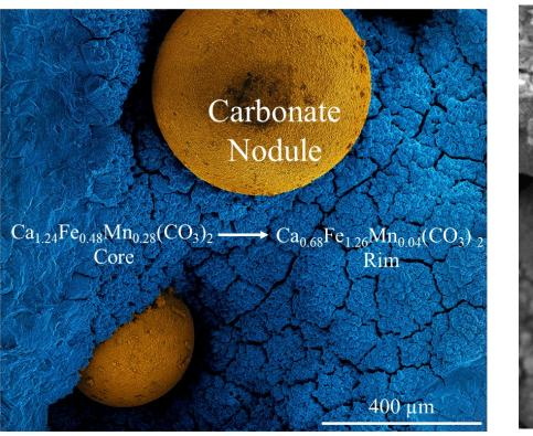
Zoned carbonate (siderite-ankerite) nodules rich in Ca, Fe, and Mn found within several sidewall cores
