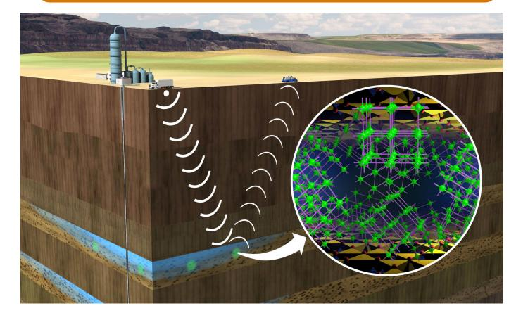
New CO<sub>2</sub> monitoring technology using seismic metamaterial contrast agents in combination with seismic imaging techniques to create a reservoir-scale periodic structure
