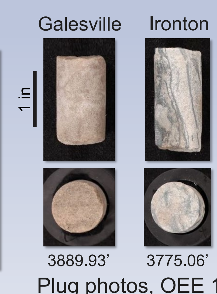
Depth 3780'-3785' Ironton core photo, OEE 1
