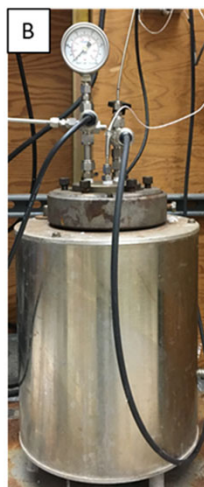
Static Autoclave System (Operability Limit: up to 250°C and 300 psi)
