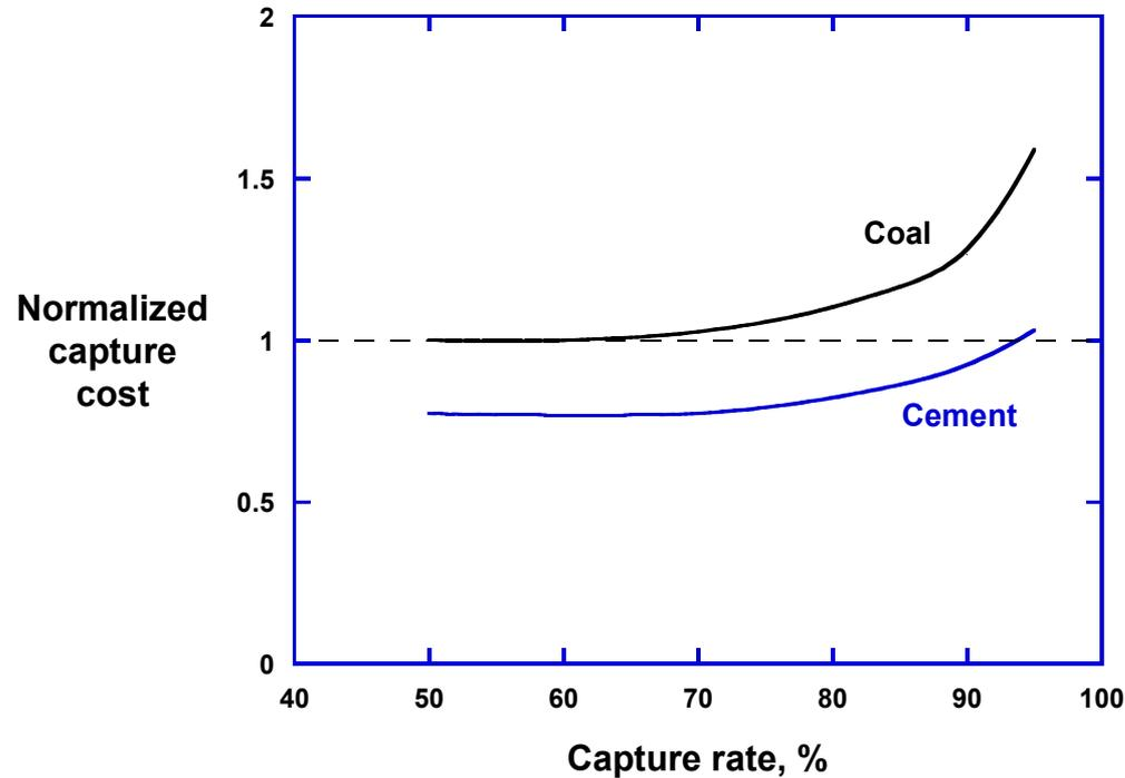
Capture cost is normalized to 60% capture from coal using today's Polaris membranes
