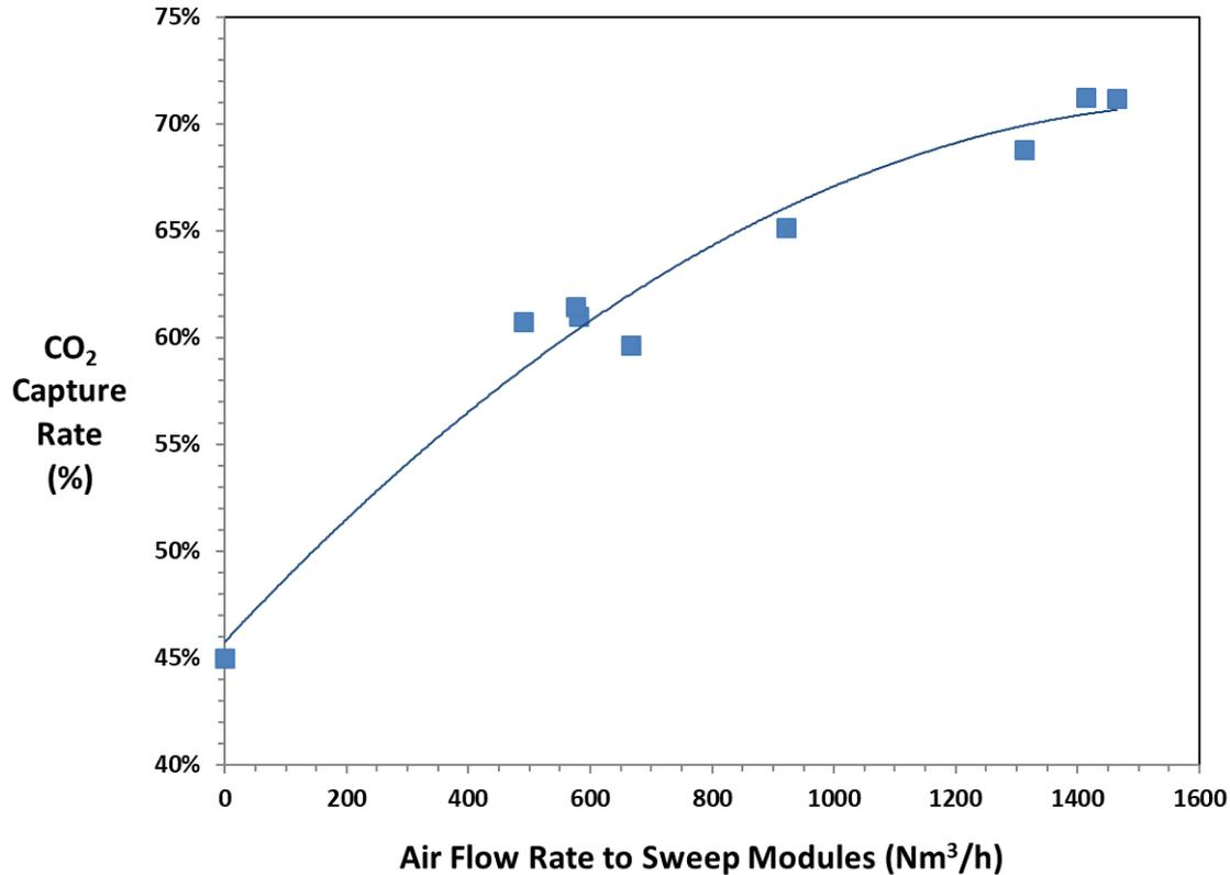
Feed = 1800 Nm<sup>3</sup>/h of ~14% CO<sub>2</sub> flue gas
