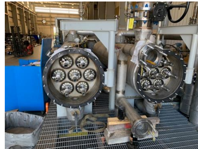
Membrane modules being loaded with new membranes prior to shipment
