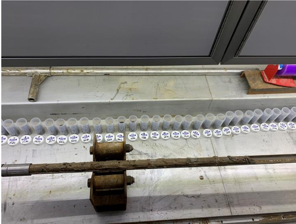
Core barrel containing continuous side-wall cores
