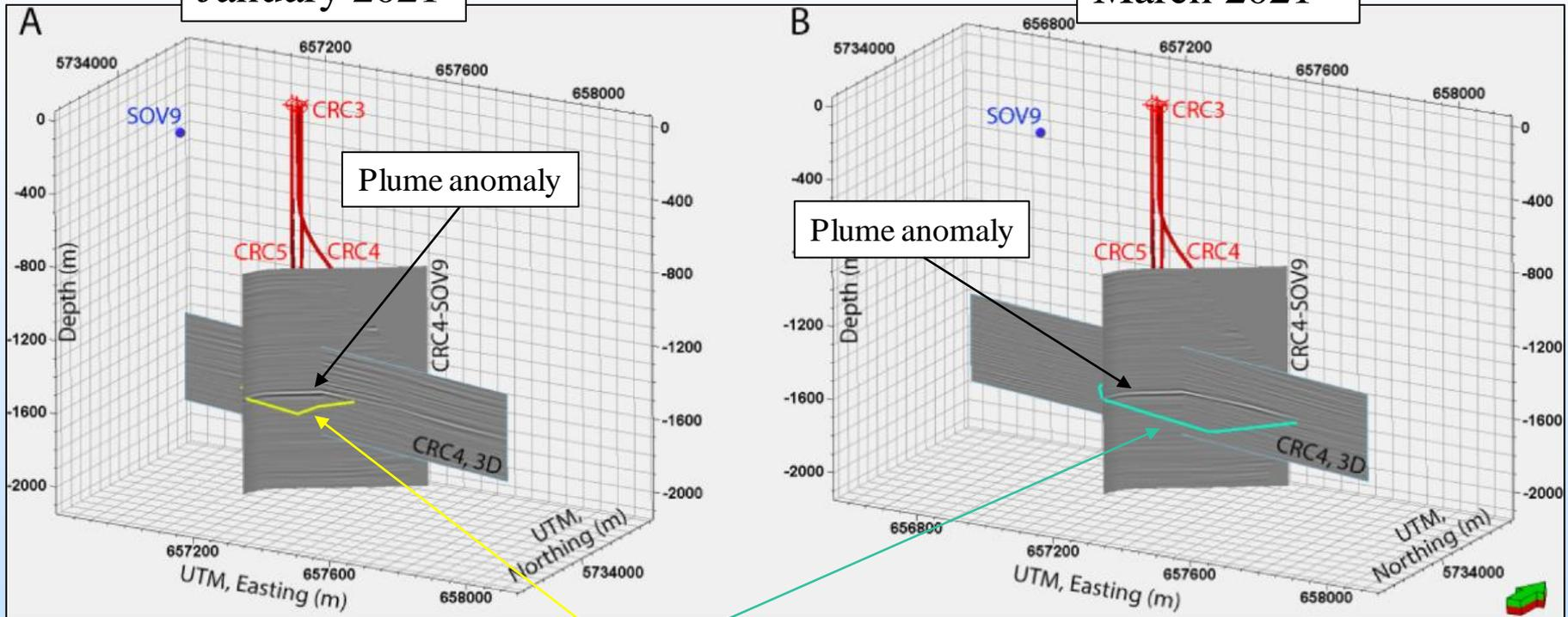
Plume contours were picked from the SOV/DAS data, before the 4D VSP seismic was acquired
