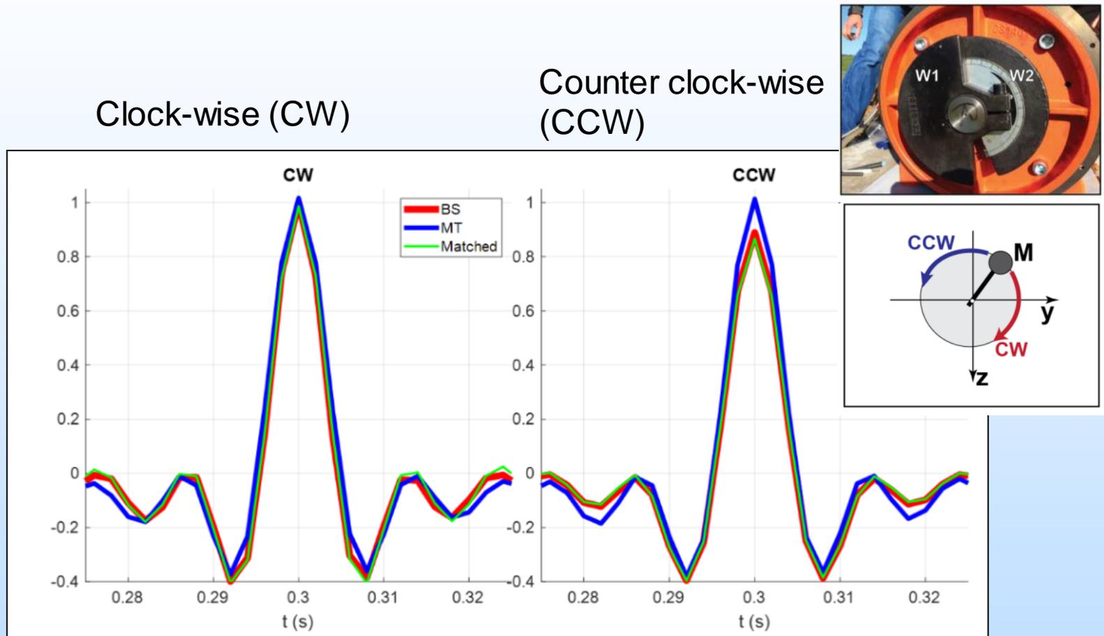
Non-repeatability of source rotation: about 10% difference in amplitude between rotations
