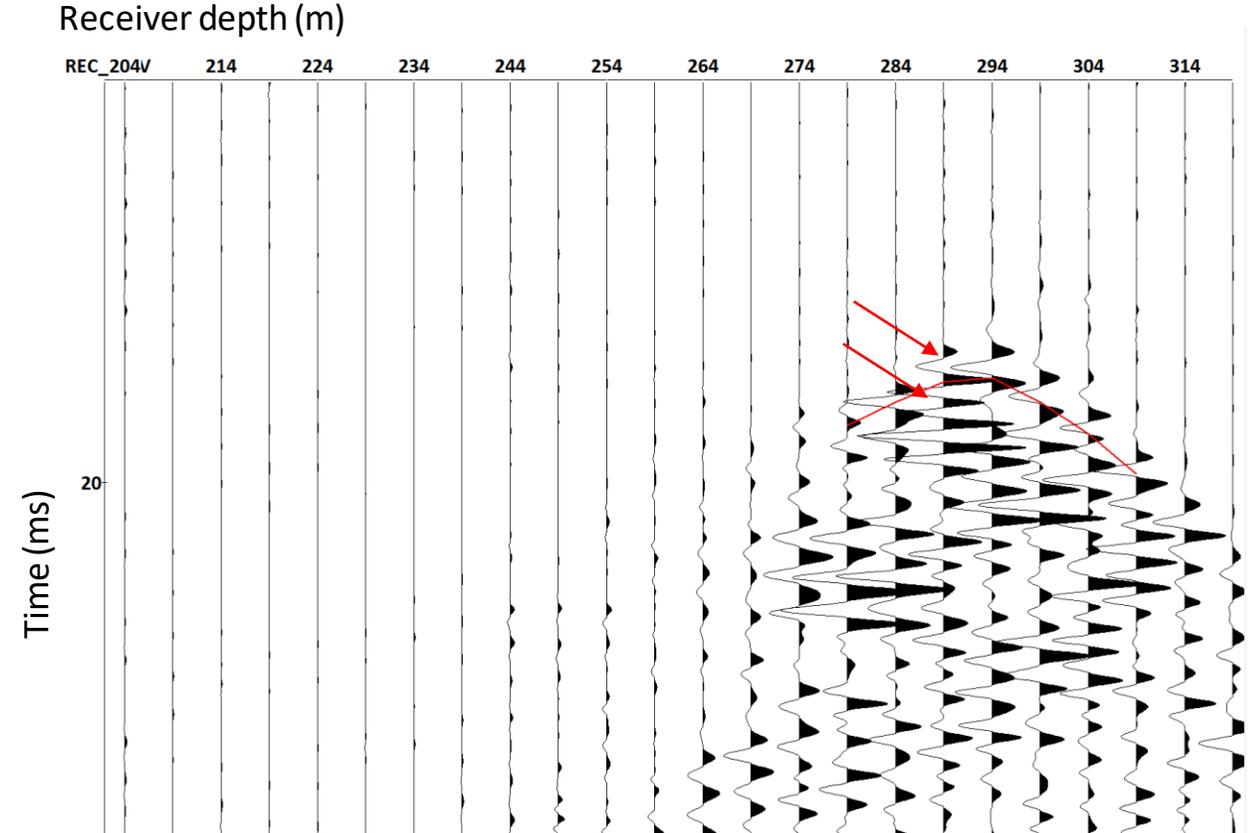
✓ Waveform differs for the two surveys + An offset-independent time delay
