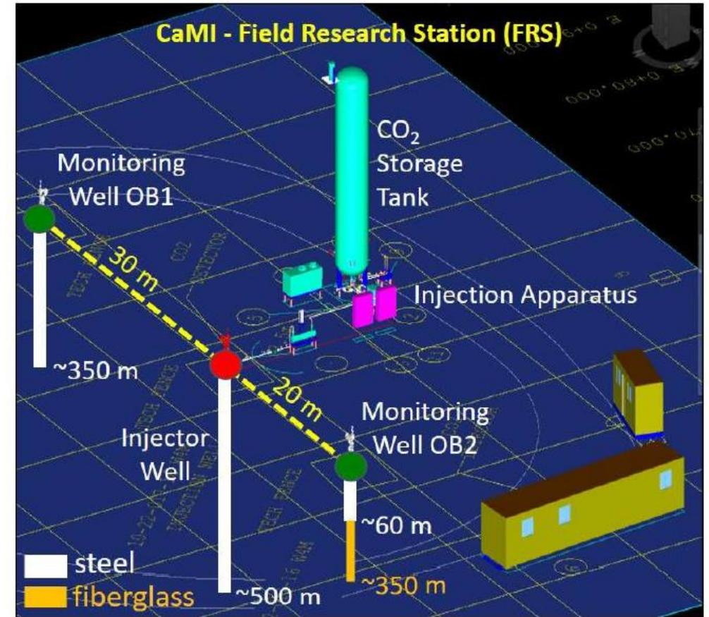
Transmitter well (Monitoring Well OB2) is highly deviated. OB1 is steel-cased, whereas OB2 is open-well (fiberglass).
