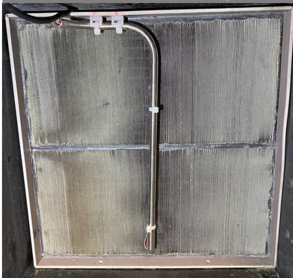
Steam outlet / air inlet, after 60 cycles
