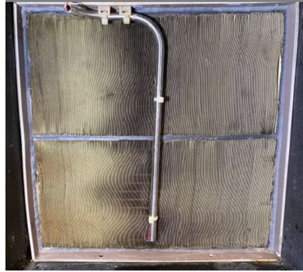
Steam outlet / air inlet, after 3534 cycles
