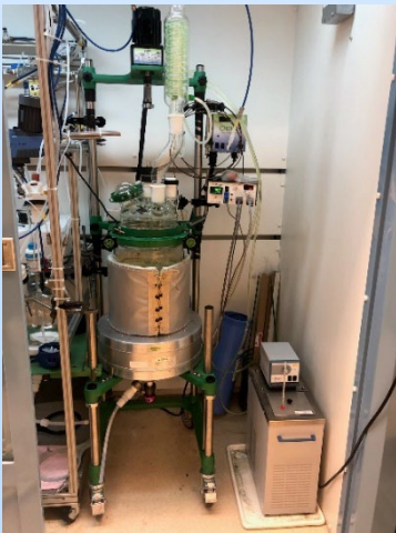
Scale up: 20L reactor
