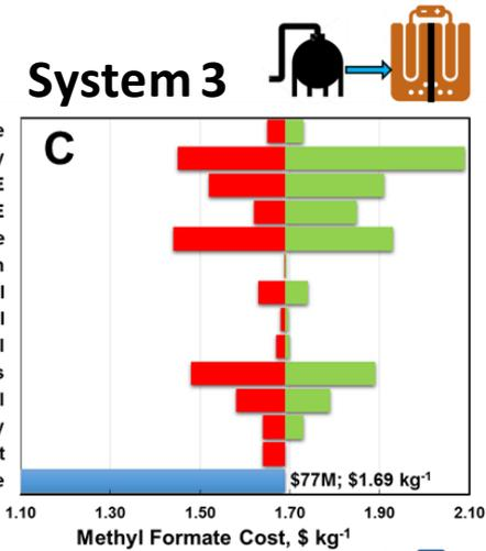
**System 3: Uses and distills twice as much CH<sub>3</sub>OH – catholyte AND anolyte**
