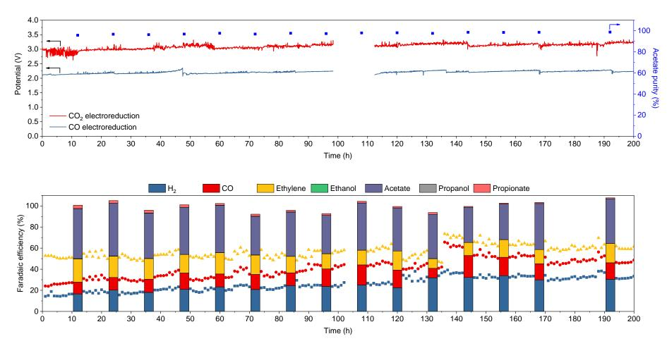
Acetate and ethylene as the main products; ~99% acetate purity; 200 hrs stability
