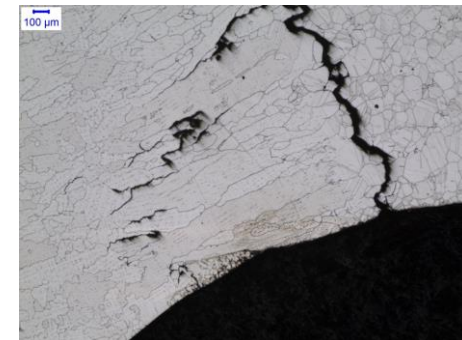
Examples of stress relief cracks initiated at weld notches
