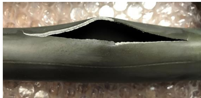
Burst test, RathGibson, North Branch, NJ
