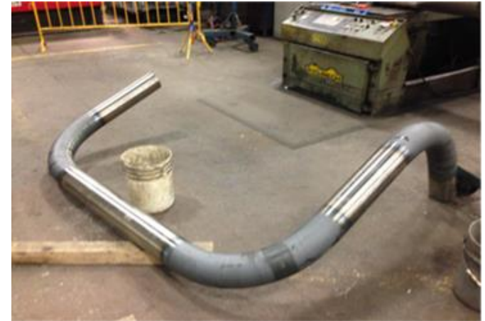
Bent and welded spool, Shaw
