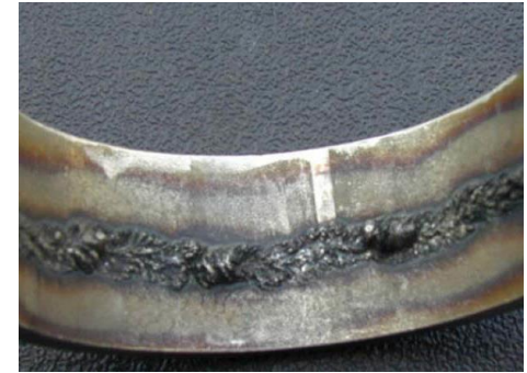
Sugaring from inadequate gas purge
