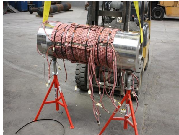
PWHT with ceramic pad, Huntington Testing
