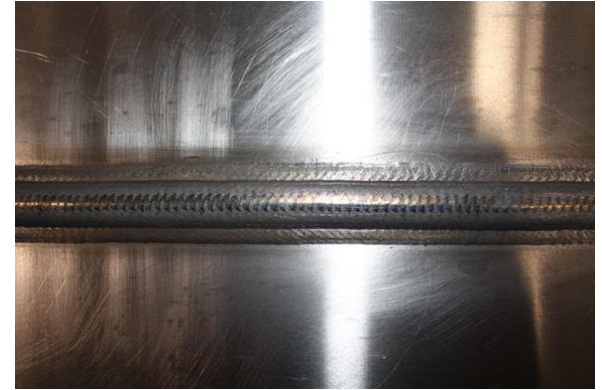
Oxide build-up on a 740H weld bead
