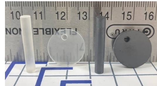
Made Yb<sub>2</sub>Si<sub>2</sub>O<sub>7</sub> and Yb<sub>2</sub>SiO<sub>5</sub> samples in collaboration with UVA (Opila's group)
