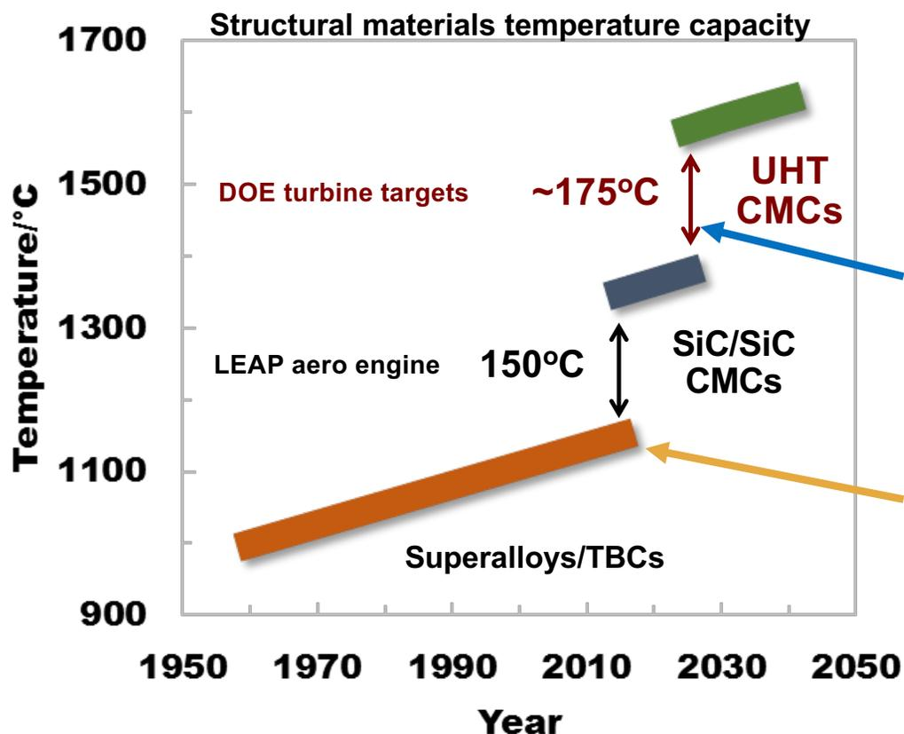
**DOE Impact:** Next generation, ultra high efficiency, utility turbines may require **~1500°C** structural materials capability AND **25,000 h** lifetime (~10X increase vs. aero applications)
