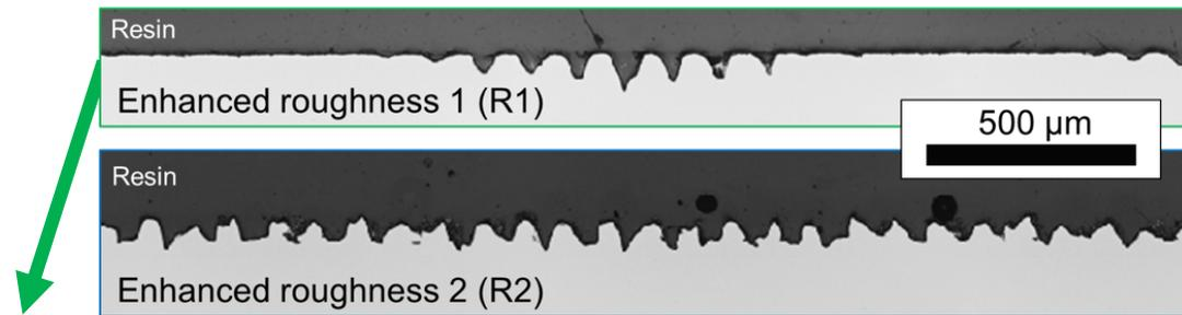
At increased roughness and ~200μm YbDS, TGO still thick and cracked
