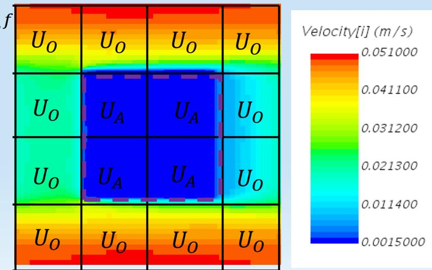
X Velocity in Cell Layer Directly above Cube from Resolved CFD
