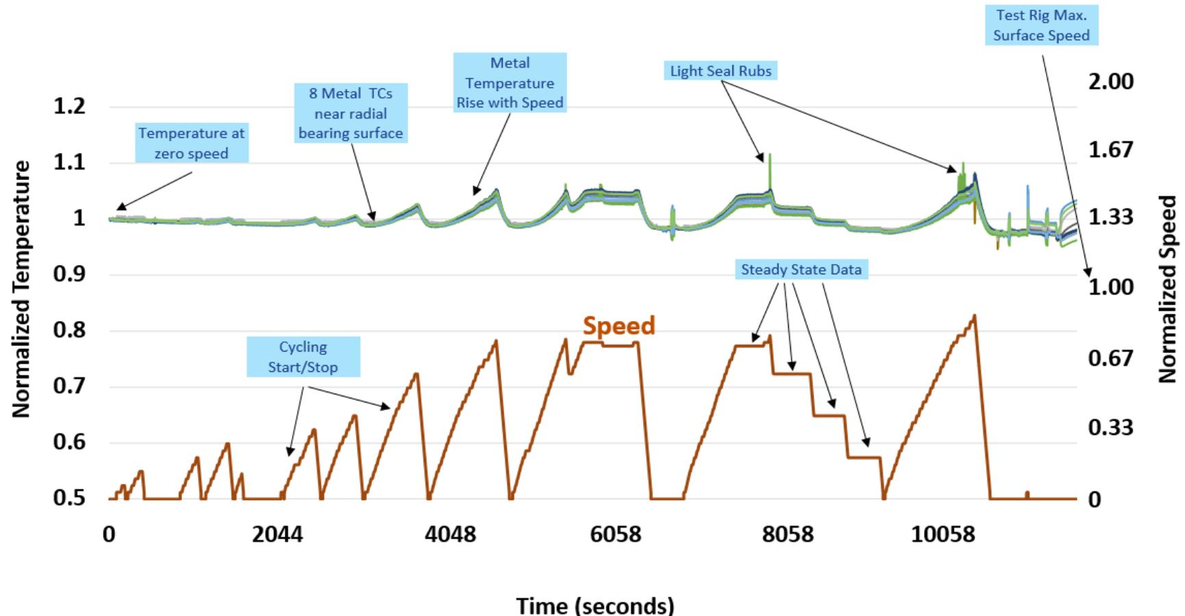
High-speed rotating tests (room temp rig) completed to successfully demonstrate TRL3 for Radial Seal Technology
