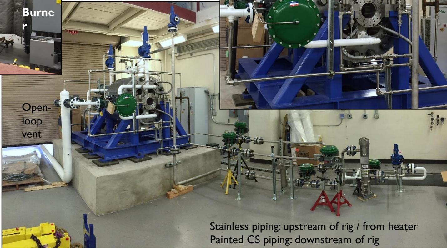
Stainless piping: upstream of rig / from heater
