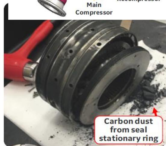
Carbon dust from seal stationary ring
