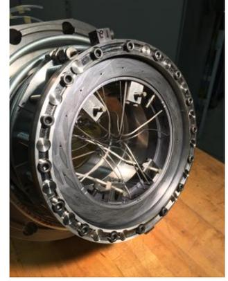
Split Seal demo in air, Low leakage ~0.45 mils, excellent match with design tools
