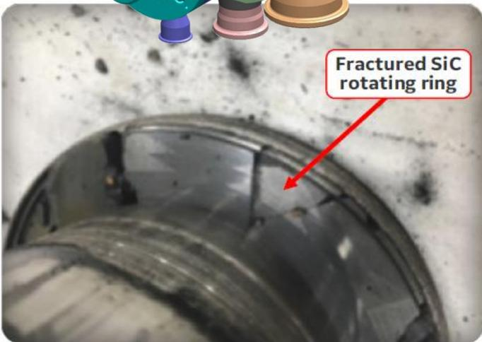
Fractured SiC rotating ring
