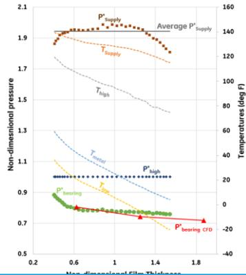
Hydrostatic lift with sCO<sub>2</sub> working fluid, excellent match with CFD
