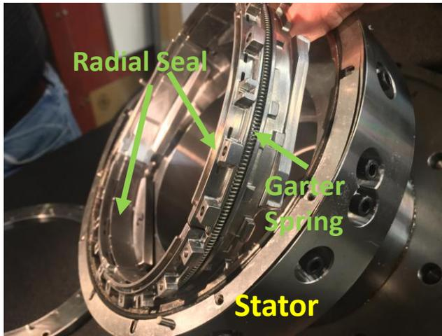
Seal Assembly with Rotor
