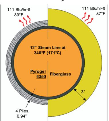
Less than 1" of aerogel-based insulation is equivalent to 3" of fiberglass. The aerogel-based insulation also requires 20% less cladding and binding
