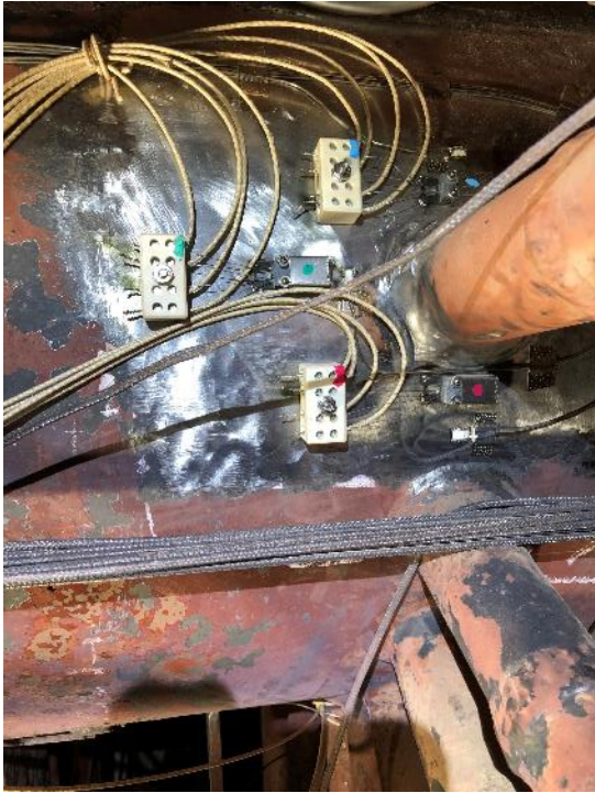
Strain Gage Installation Near Assembly 25 SCST
