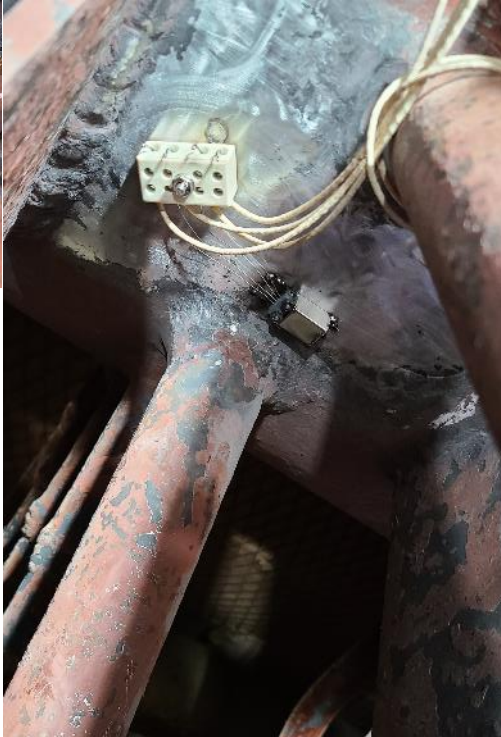
Strain Gage Installation SSOH Header Bottom
