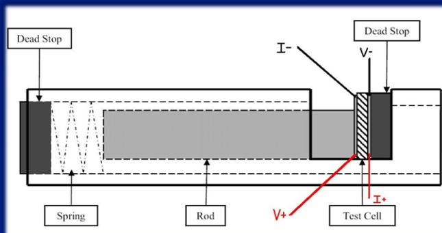
Schematic of ASR Test Cell
