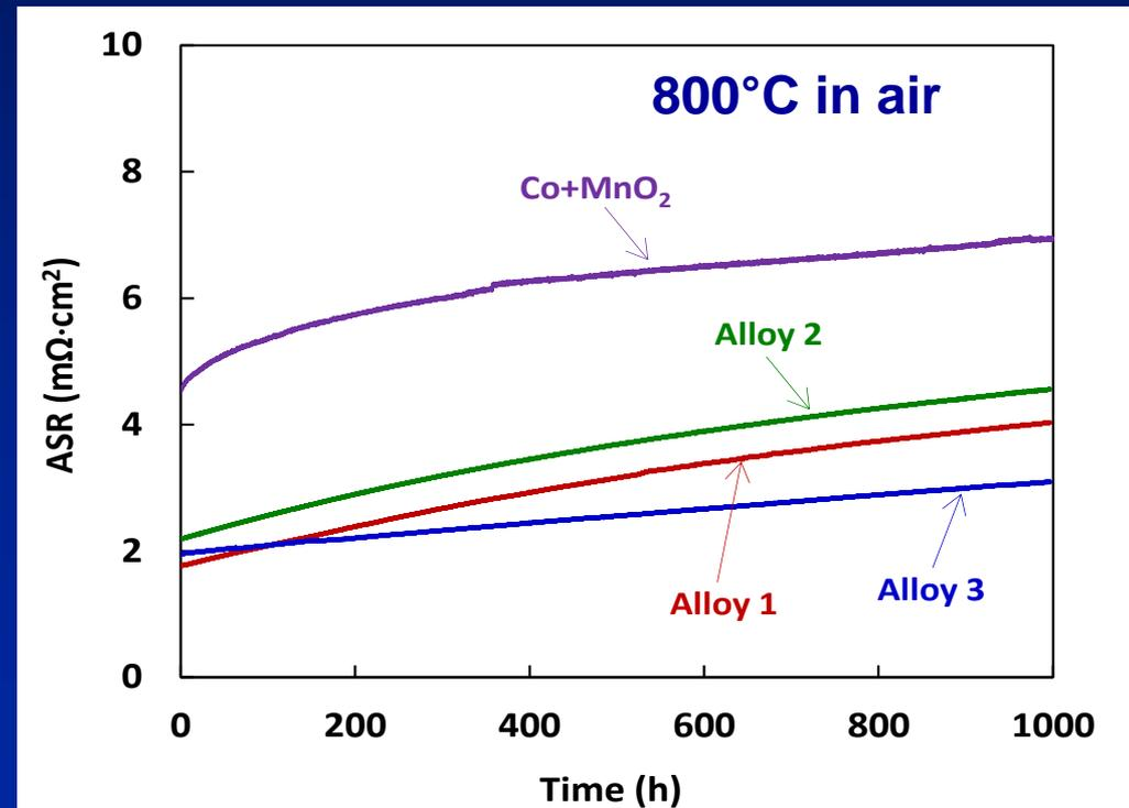
Cell ASR vs. Time of Test Cells
