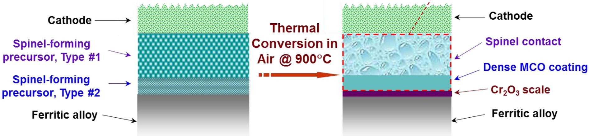
Schematic of Co-sintering of Spinel-Based Coating/Contact Dual-Layer Structure<sup>17</sup>
