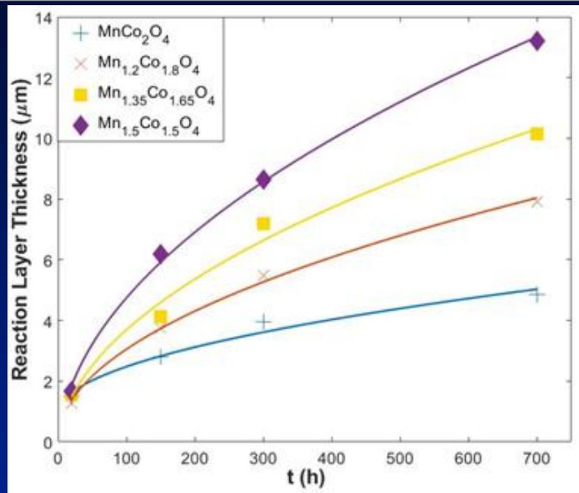
Thickness of the reaction layer vs. t
