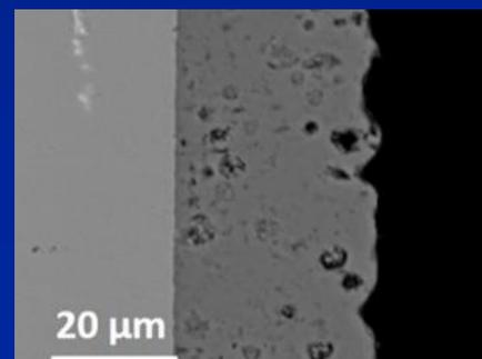
Cross-sectional View of Converted Alloy-1 Layer
