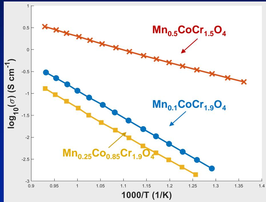
Electrical Conductivity vs. 1/T of Different Reaction Layer Compositions
