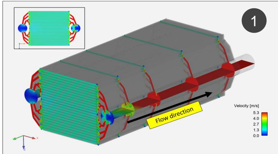
1. Stack CFD model has been developed to predict the cell-to-cell flow distribution across the stack consisting multiple fuel cells.
