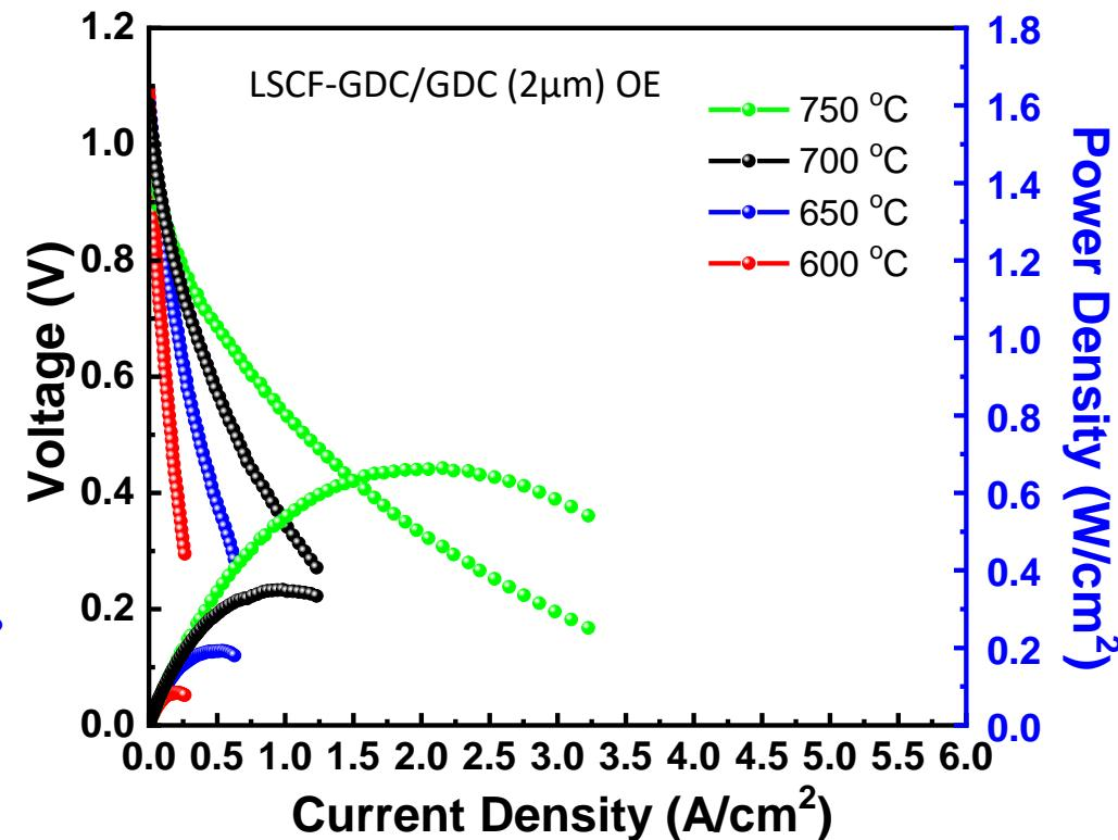
HE substrate: 300  $\mu\text{m}$  ScSZ-Ni; HE functional layer: 10  $\mu\text{m}$  ScSZ-Ni;
