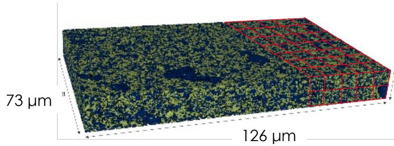
3D Reconstruction of SOFC Electrodes
