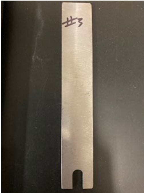
Stainless steel beam
