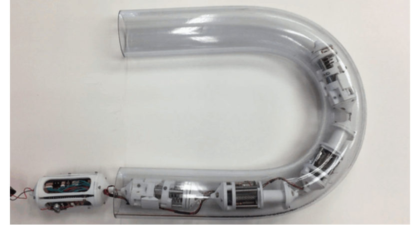
180-degree Bend test
