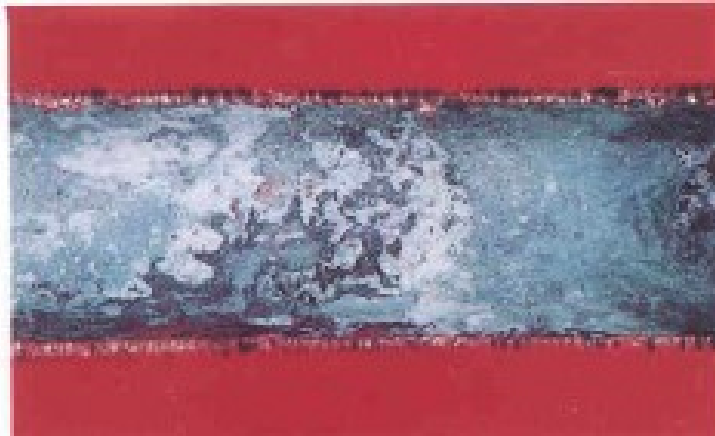
General corrosion inside copper tube because of CO 2
