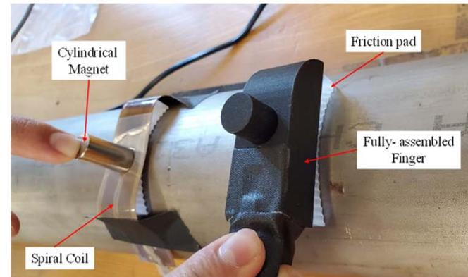
For diameter larger than 3" the 1mm lift-off resulted in acceptable SNR
