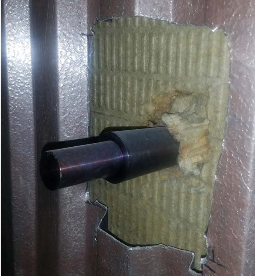
Waveguide welded to waterwall's membrane; shown after the waterwall was covered with insulation
