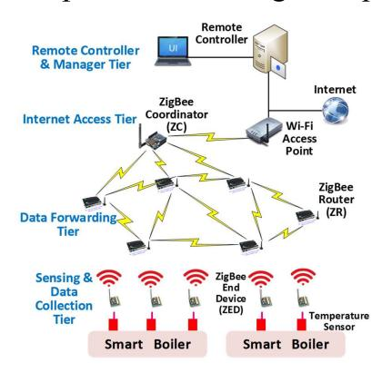
High-temperature WSN testbed
