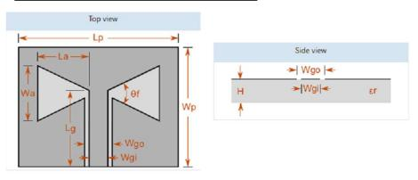
Antenna design parameters using Antenna Magus and CST Microwave Studio®.
