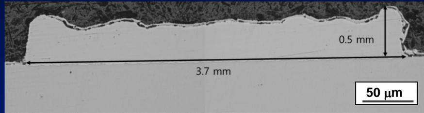
H282 deposited using Purdue's powder bed fusion (PBF) system
