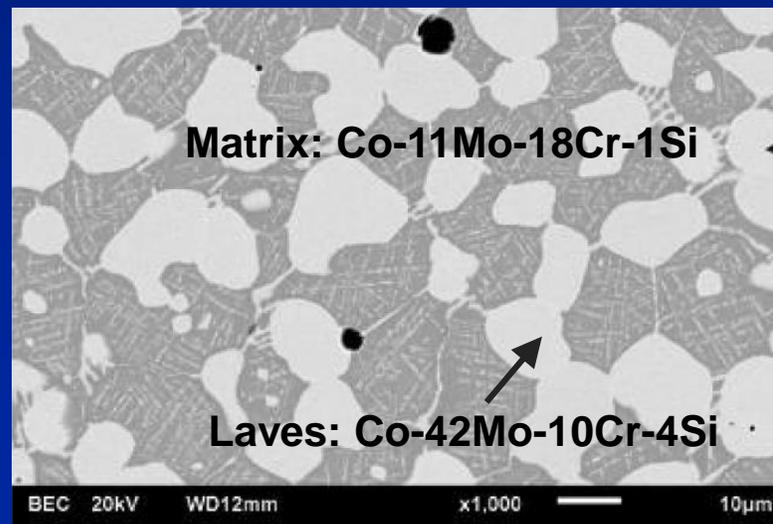
**Cr:** corrosion/oxidation resistance
