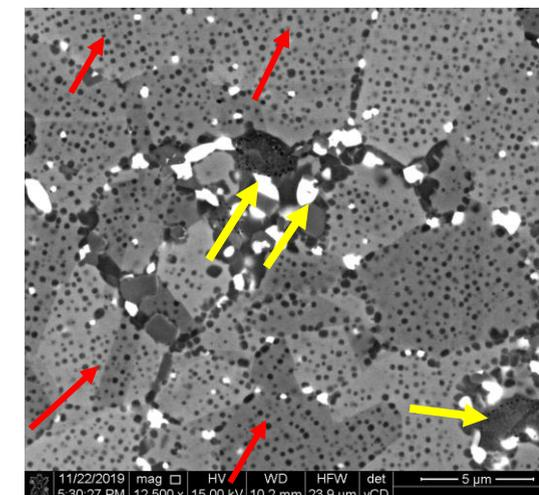
**FSP + 2 step heat tx + 500 hrs @ 871°C**
