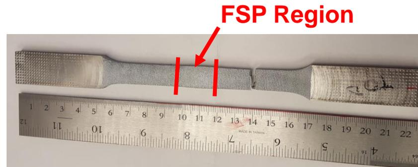
Room Temperature Tensile Test Coupon
