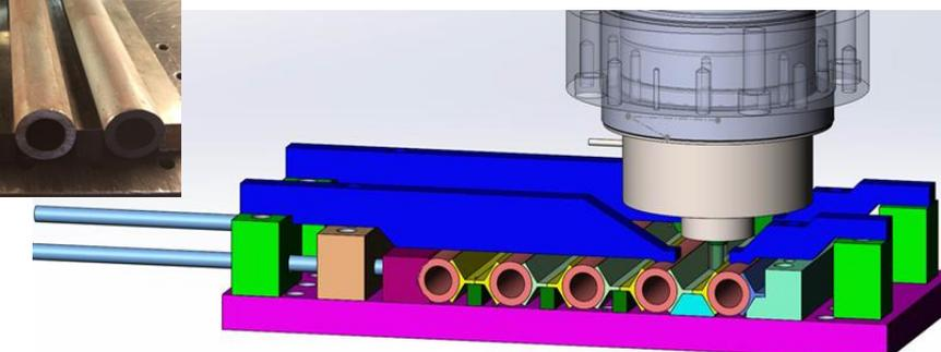
Membrane Wall Friction Stir Welding
