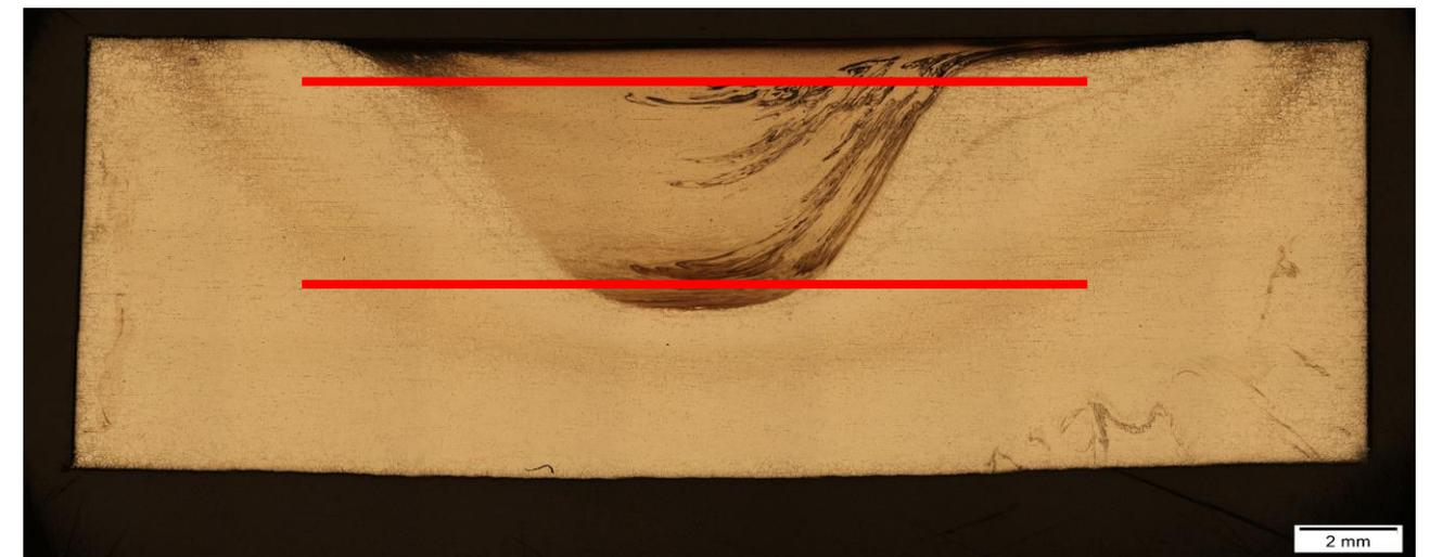
Creep Testing Coupon Material Area
