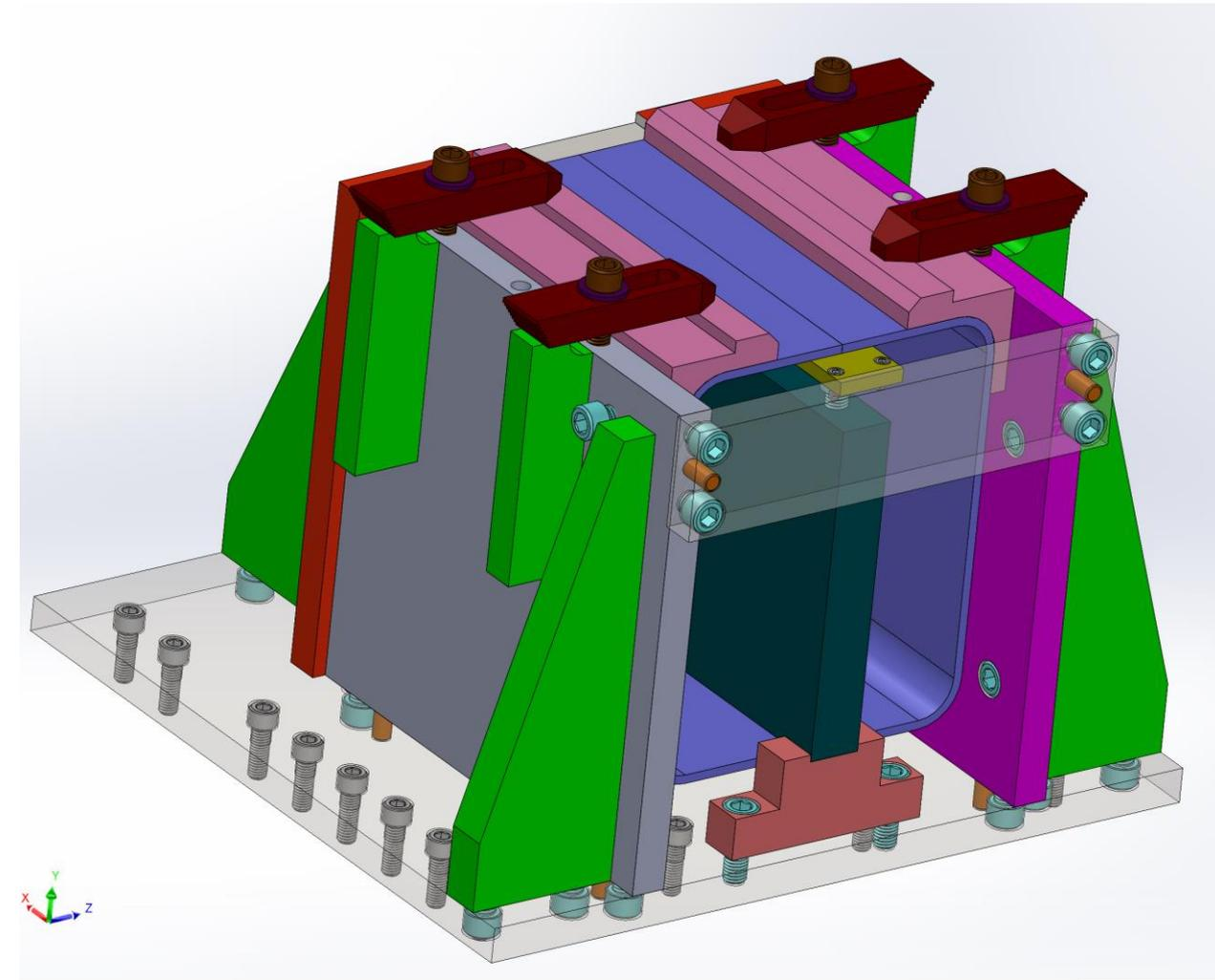
**FSW Fixture with Prototypic Part**
