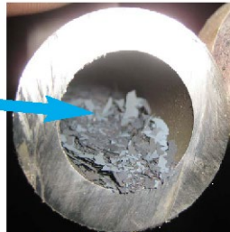
Spalled oxide scales cause pipe blockage
