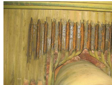
Corrosion fatigue damage in the steam-cooled wall where cycling caused differential thermal growth
