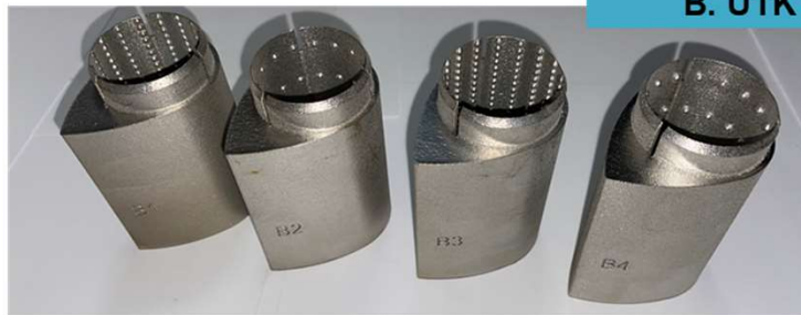
C. Siemens dual thermal flow topology optimized ext. surf design
