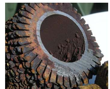
HRSG feedwater heater tube leaked from cold-end corrosion during cycling.
