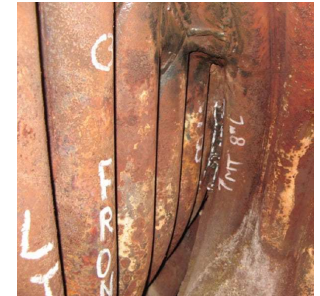
Waterwall corrosion fatigue damage due to cycling damage at a corner
