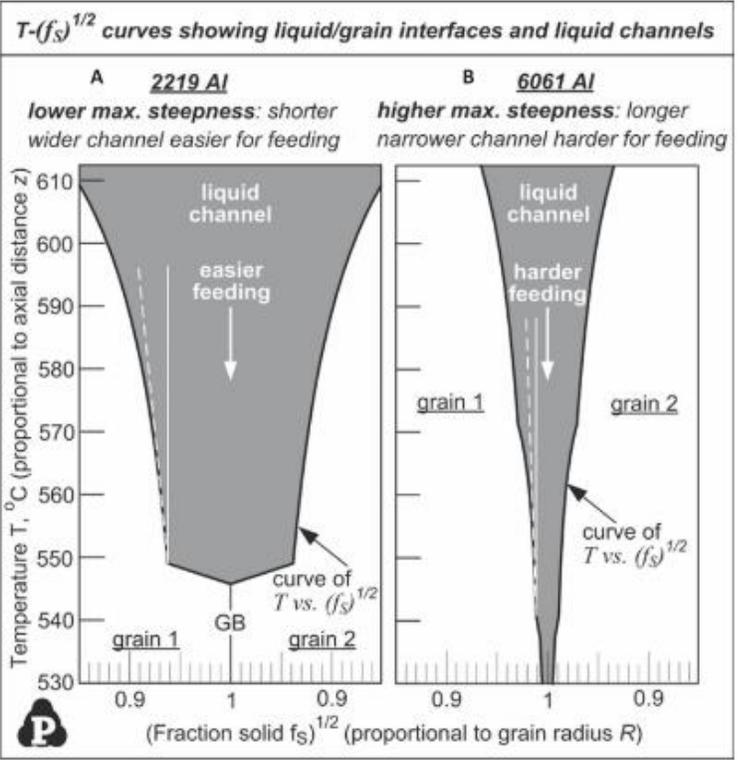
Fig. 12 —  $T-(f_s)^{1/2}$  curves showing liquid/grain interfaces, liquid channels and tangents to curves at locations of maximum steepness. A — 2219 Al alloy; B — 6061 Al alloy. A longer, narrower channel hinders liquid feeding because of the resistance to flow caused by the viscosity of liquid.
