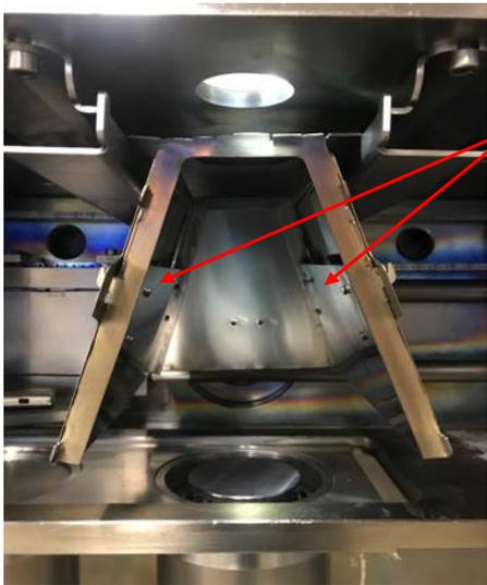
Stainless steel plates used as backscattered electron detectors (BSE)
