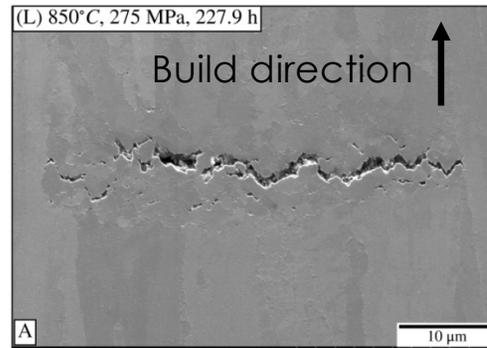
AM materials can contain heterogenous 'stray grains' which crack during creep
