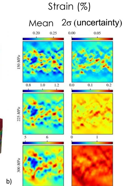
Creep properties anisotropy likely related to crystallographic texture and heterogenous stray grains leading to local stress concentration
