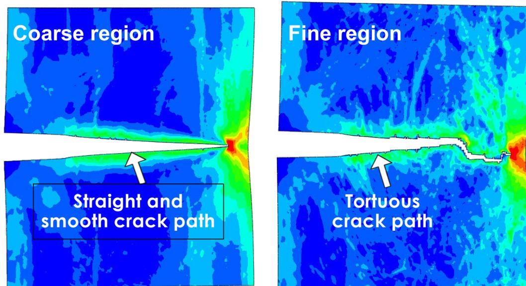
CPFEM simulated crack path
