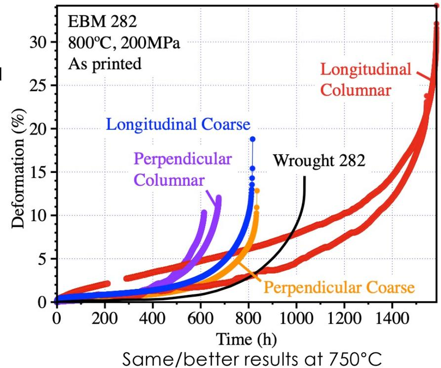
Superior creep strength with columnar grains along the build direction (BD) but significant creep strength decrease perpendicular to BD
