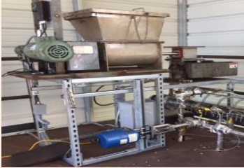
Coal hopper & volumetric feeder
