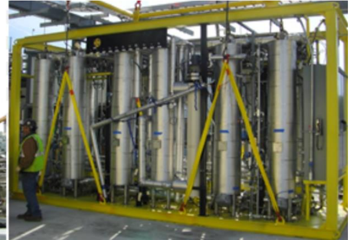
TDA 0.1 MW pre-combustion carbon capture unit installed at the National Carbon Capture Center
