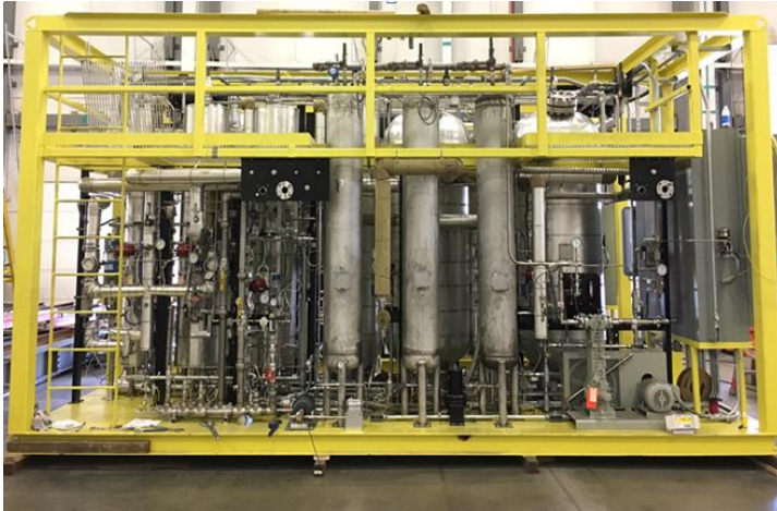
TDA 0.1 MW pre-combustion carbon capture unit installed at the National Carbon Capture Center
