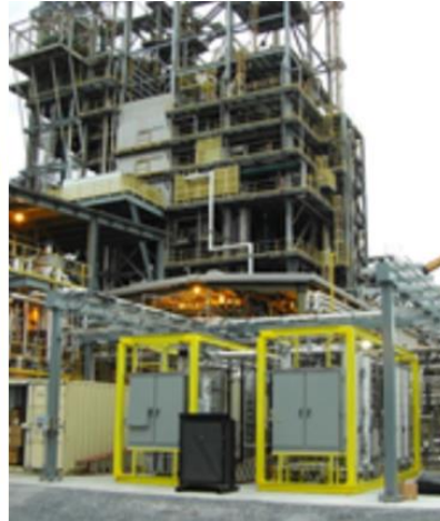
TDA 0.1 MW pre-combustion carbon capture unit installed at the National Carbon Capture Center
