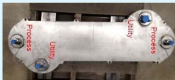
Double-Sided Absorber – Combined Sorption and Desorption Cycles Integrate heat of sorption with heat of desorption.
