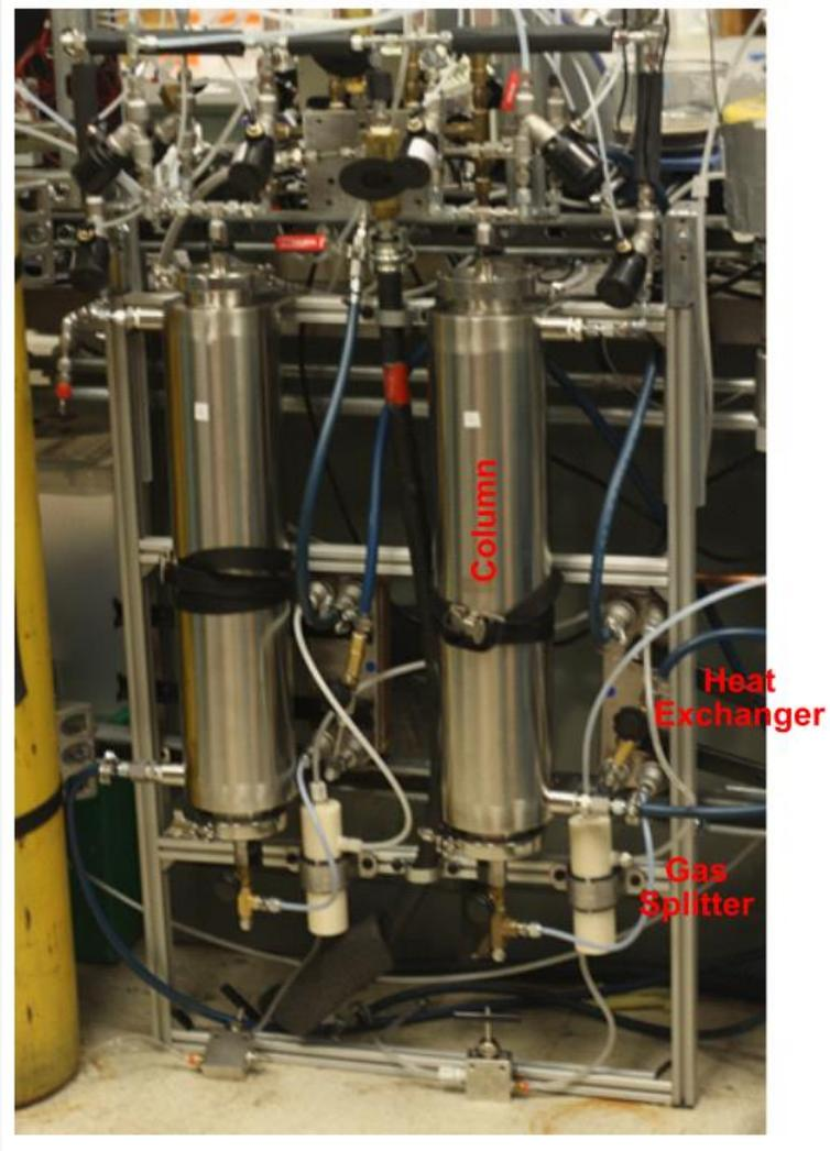
Gemini apparatus for sorbent testing
