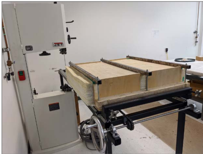
Membrane module stack trimming system
